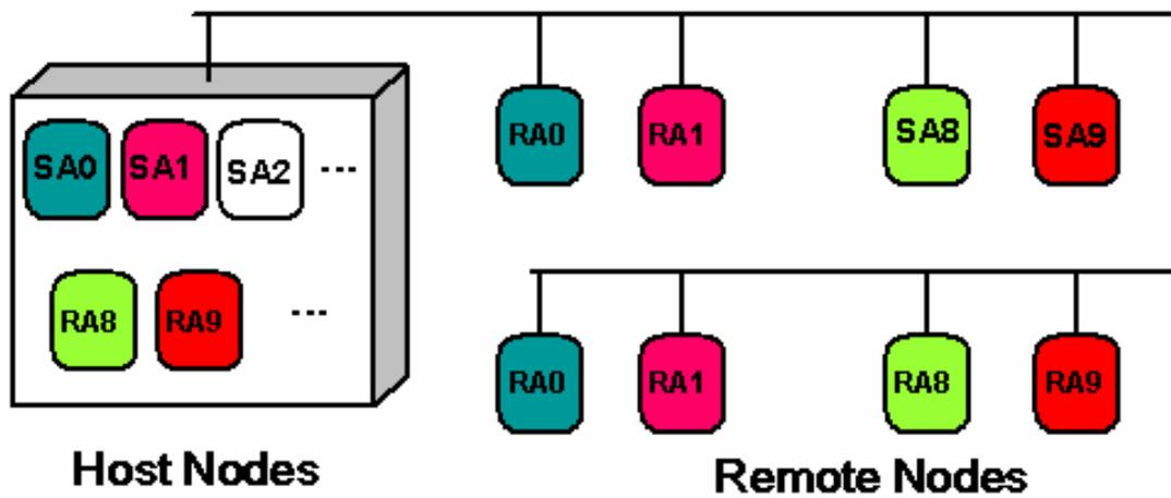
Figure 1.2 The example of an FRnet application structure
