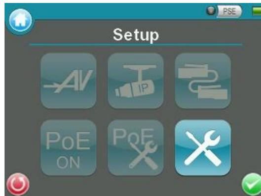
Step 2: Tap <Setup- IP>
