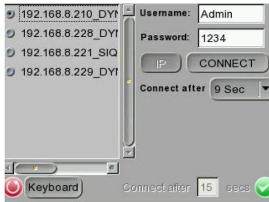
Tap <IP/MAC> to switch the detected IP Camera displaying form between IP address and MAC. Select the target IP Camera from the device finding list on the top left of the screen. And setup the duration to wait until connecting to devices. For a custom setting, select <Custom> from the drop-down list and then enter the value in the field at the bottom of the setup page. Then tap <CONNECT> beneath the Password column to start connecting. The live view video will be displayed on the screen.
