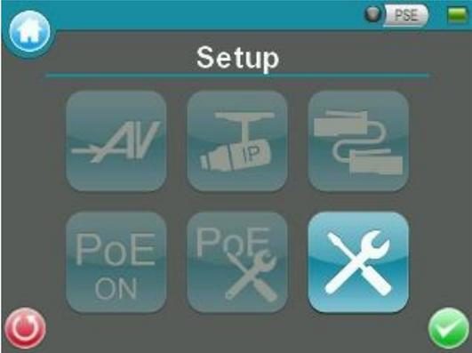
Step 2: Tap the <Setup- System>
