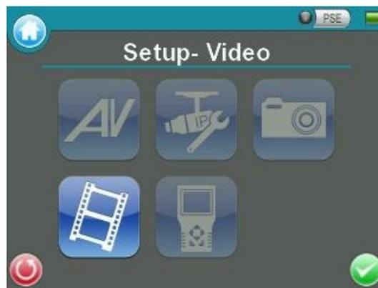
Step 2: Tap <Video- Rec setup>
