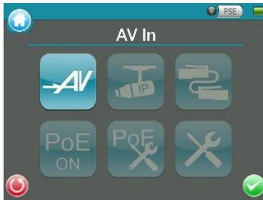
**NOTE:** To view live video from an IP Camera which supports BNC via AV In function, please make sure the IP Camera streaming is set as “BNC Out”.
