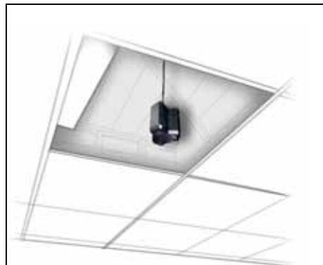
Installation of Omni-Masking Speaker (OMS) in Ceiling Plenum
