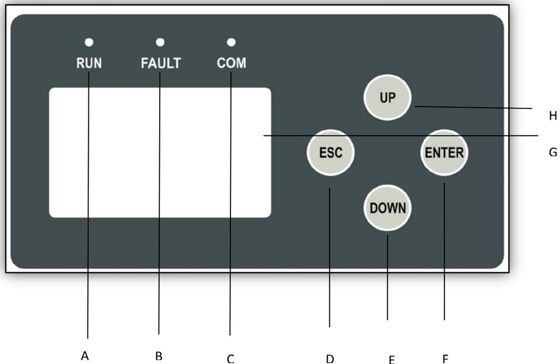
Figure 5-1 Control and Display Panel
