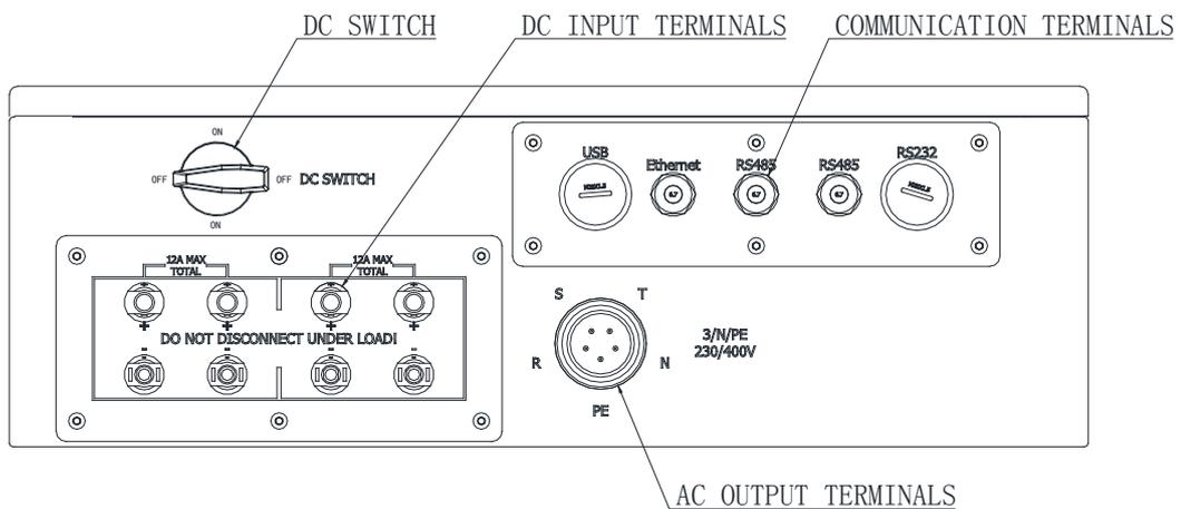
Figure 2-2 Electrical Terminals of TRI010KTL
