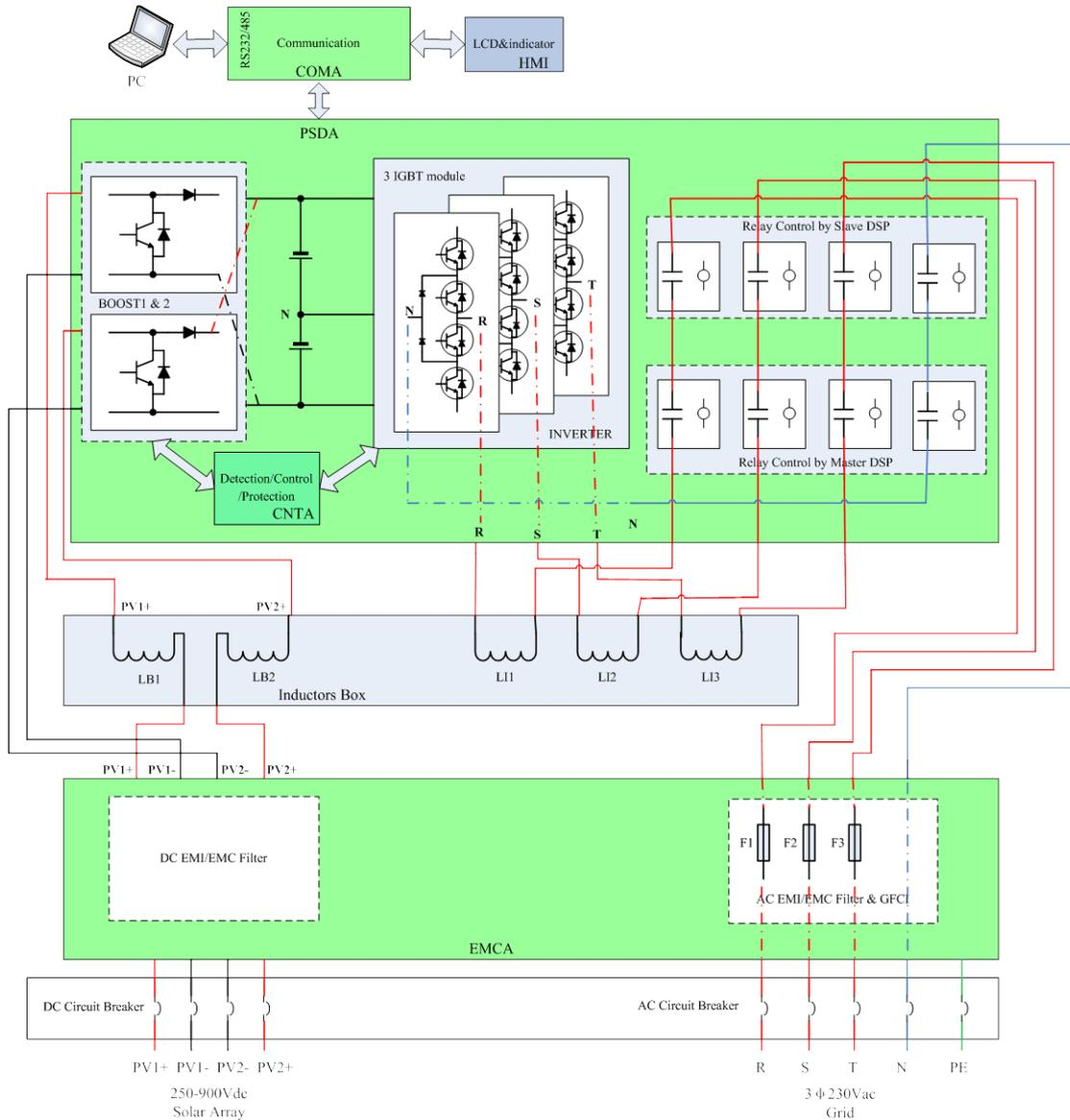
Figure 2-5 wiring diagram of the whole TRI010KTL/012KTL/017KTL/020KTL system
