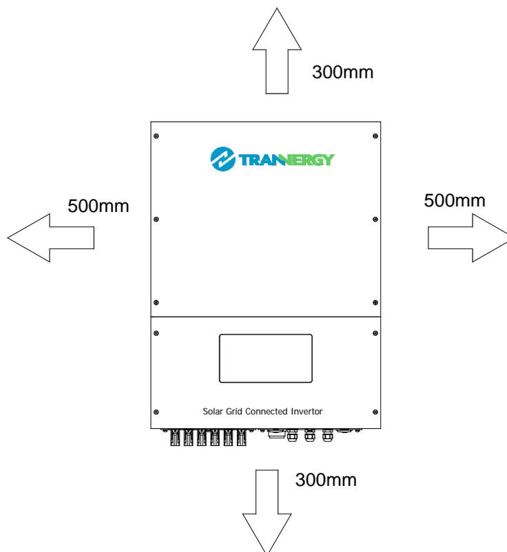
Figure 4-1 Distance required of Invertors
