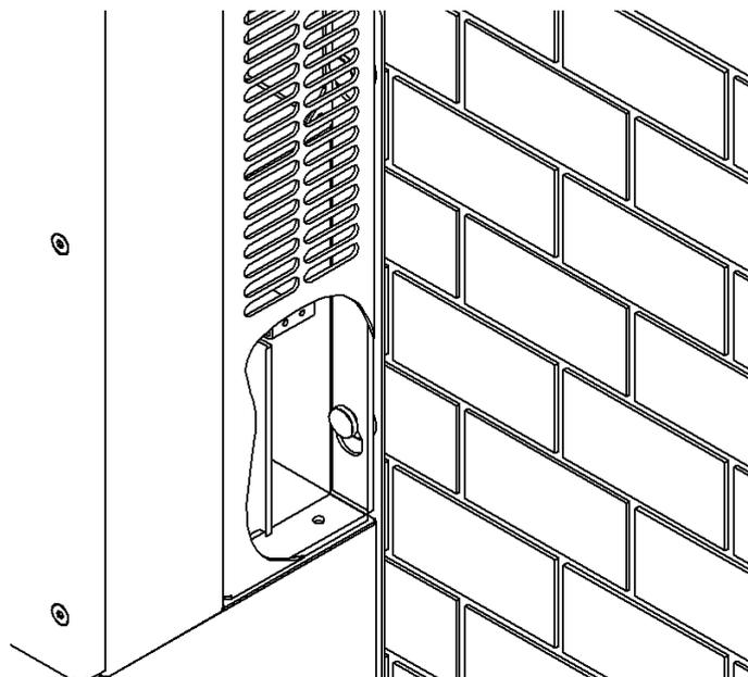
Figure 4-5 Hung the inverter
