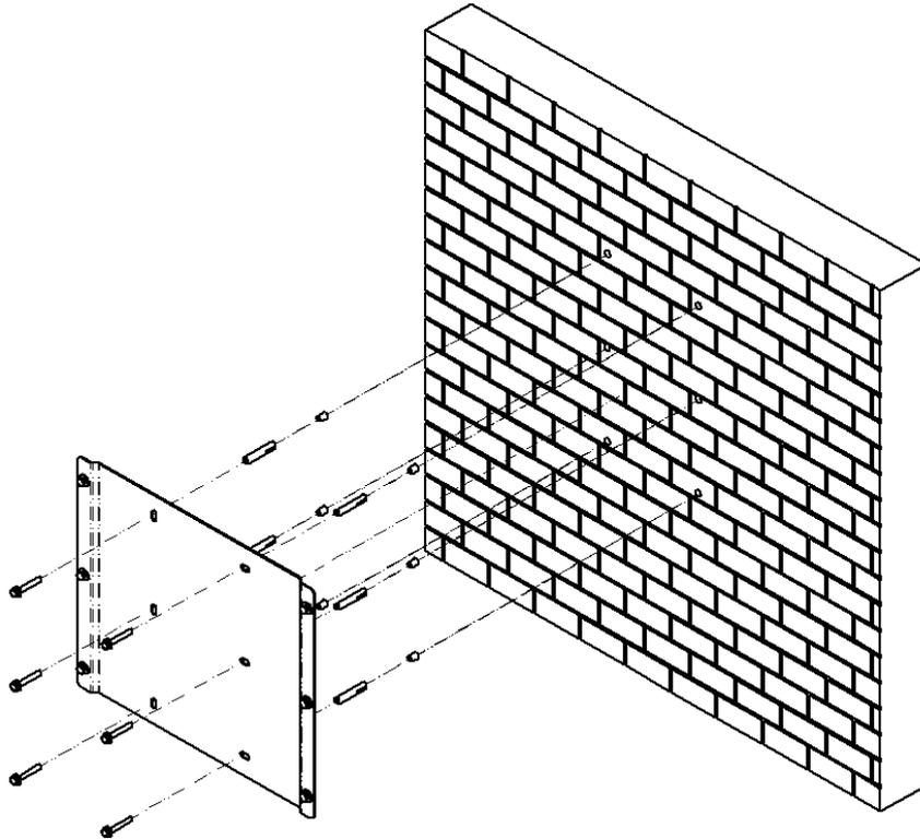
Figure 4-4 Install the mounting panel
