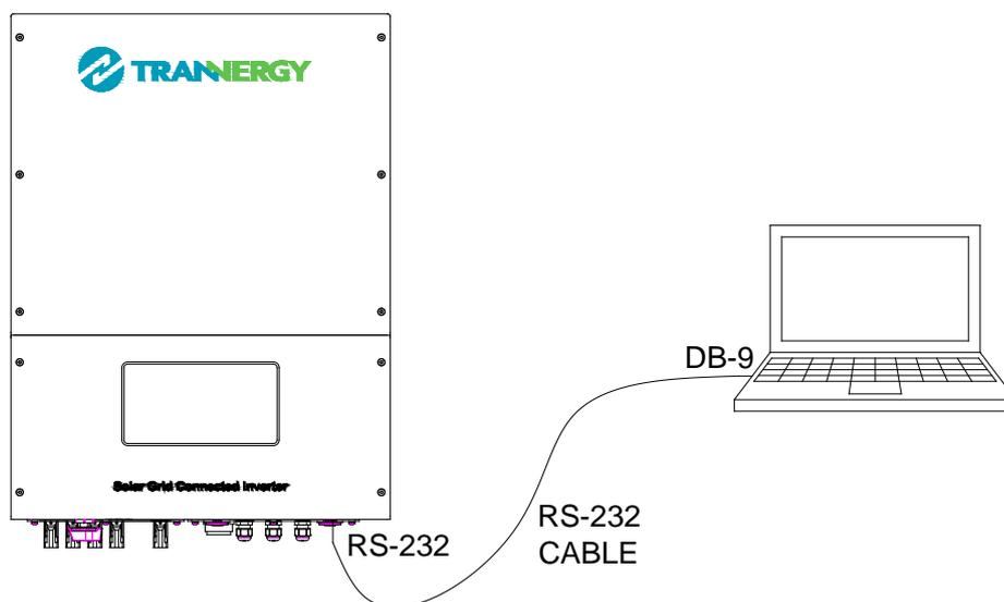
Figure 6-1 RS-232 Communication Diagram
