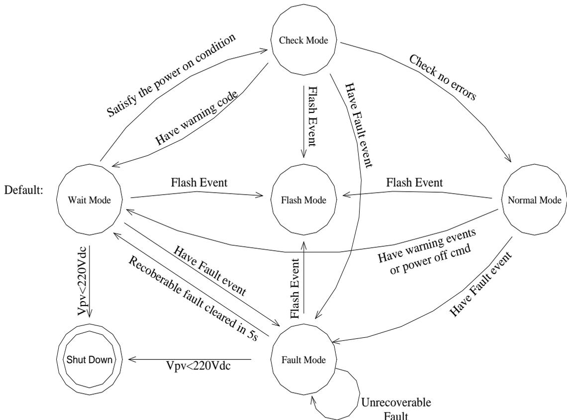
Figure 3-1 State Machine of Inverter working mode
