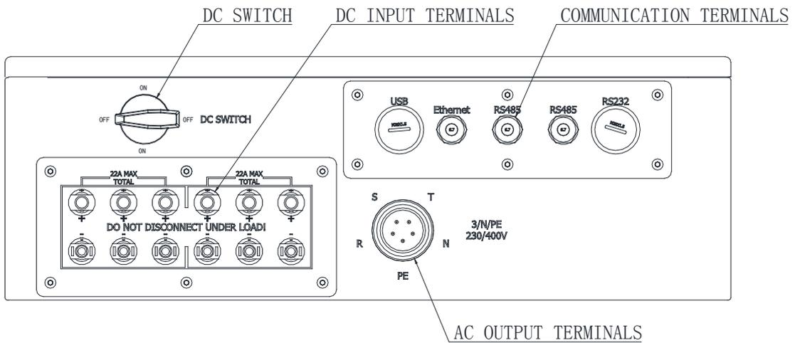
Figure 2-4 Electrical Terminals of TRI017KTL/020KTL
