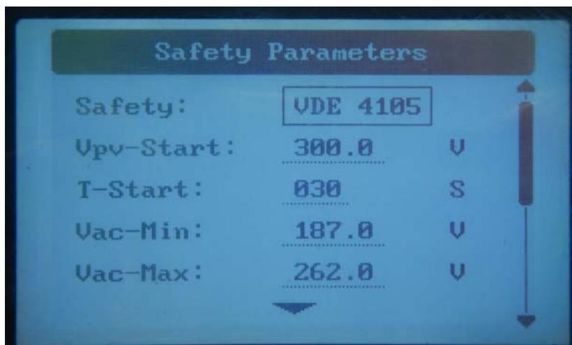
Figure 5-8 Safety Parameters Setting
