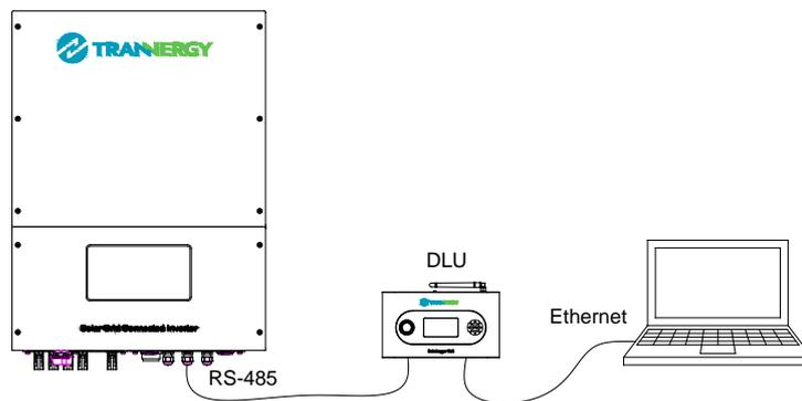
Figure 6-2 RS-485 Communication Diagram
