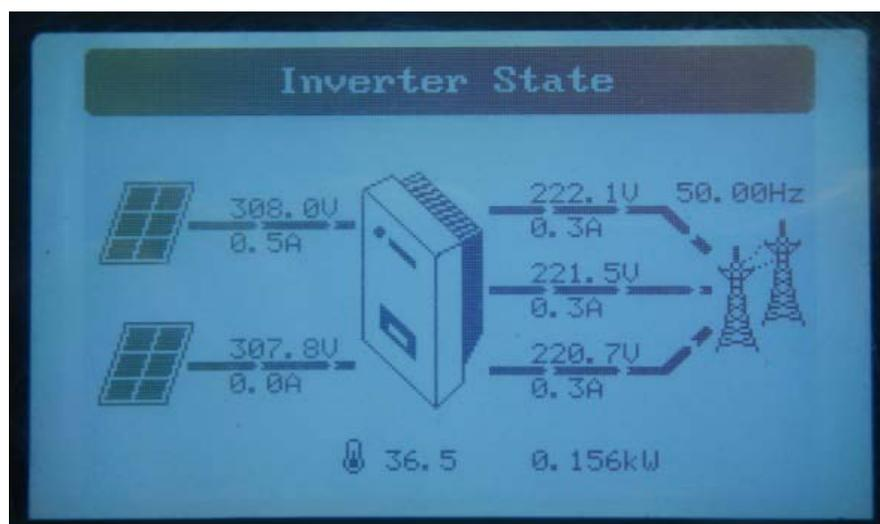
Figure 5-13 Inverter state Interface
