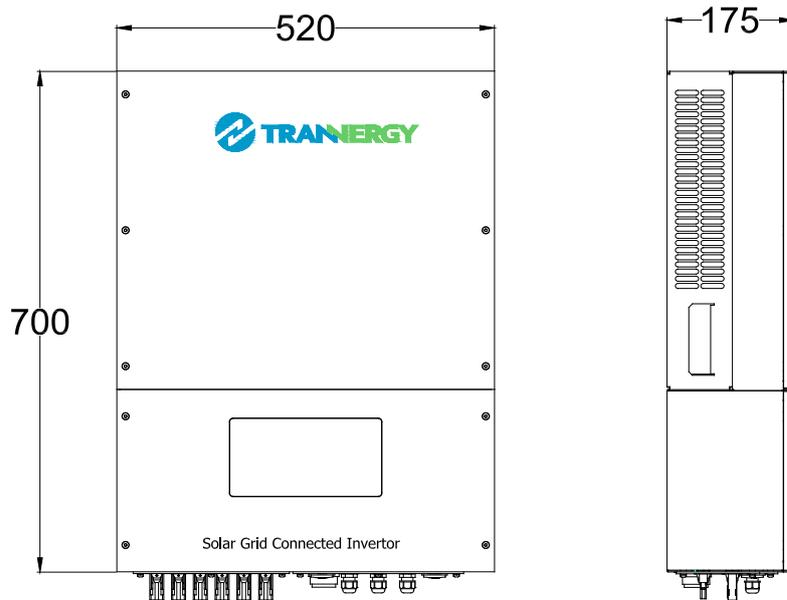
Figure 2-1 Outline dimensions of TRI010KTL/012KTL/017KTL/020KTL
