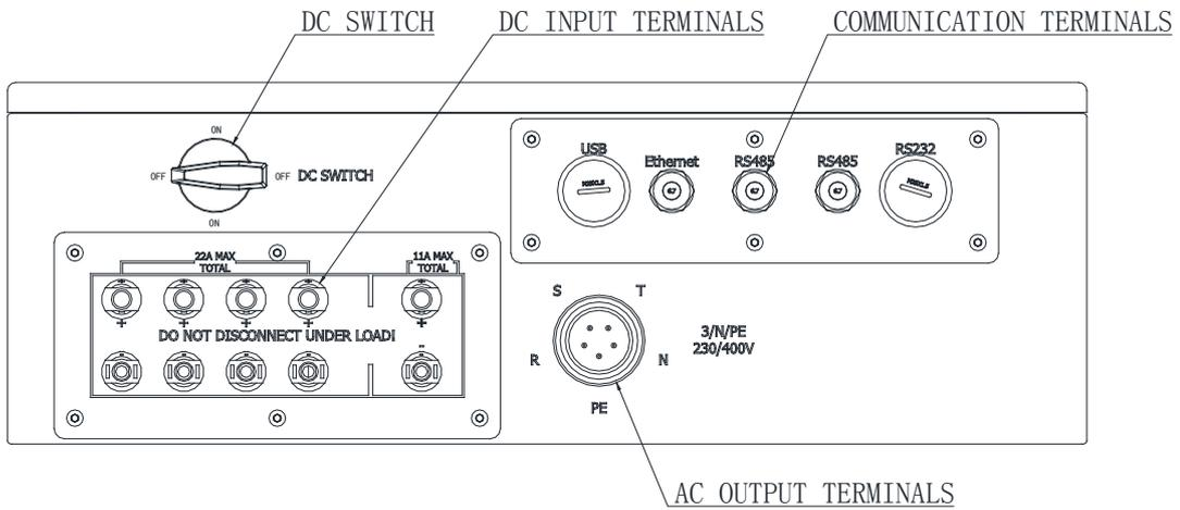
Figure 2-3 Electrical Terminals of TRI012KTL
