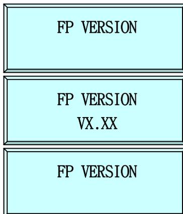
☞ . To check what version of Fingerprint(FP) module is installed to the device, press <ENT> key.
