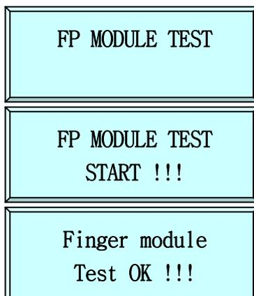
☞ . To ensure that the installed fingerprint module is operating without any problem, press <ENT> key.
