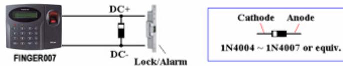
Figure : Reverse Diode connection
