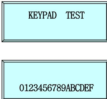
☞ Press <ENT> key to start the keypad test. When operating normally, pressing the keys on the keypad will display the corresponding letter on the LCD.
