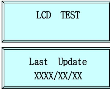
☞ To test the performance of LCD, press <ENT> key. As the test proceeds several characters will move quickly from right to left.
