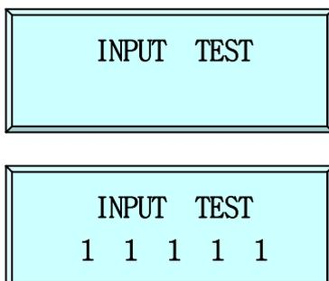
☞ To test performance of input ports, press <ENT> key. The lower line on the LCD indicates the status of the five input signals.
