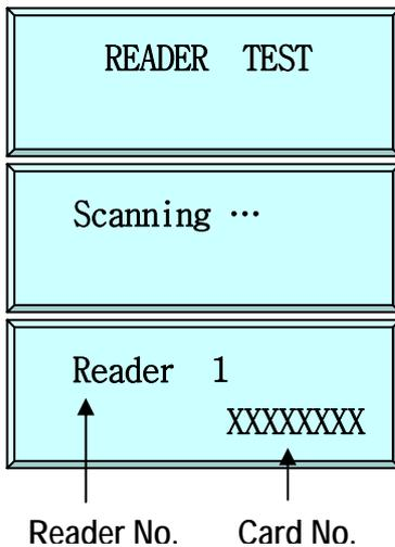
☞ To test the performance of the reader, press <ENT> key.
