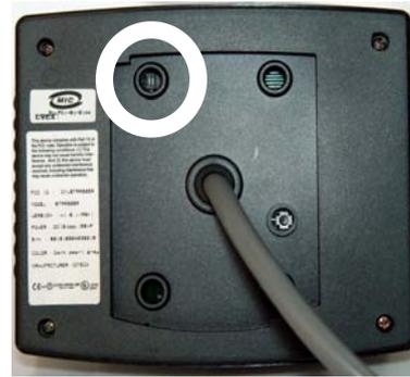
Figure : DIP Switch location
