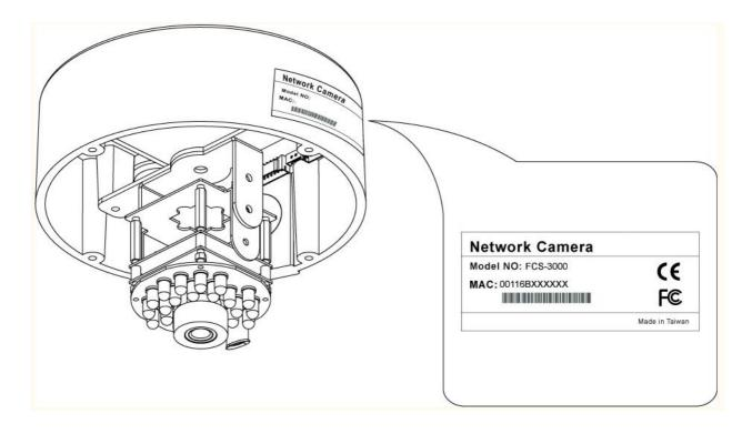
For the MAC address, please check the label on the bottom of the camera.
