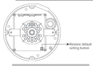
Restoring the factory defaults will erase any previous settings. Reset or restore the system after power on.
