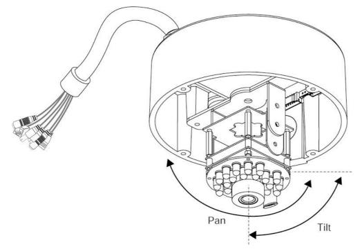
4. Use the pan/tilt mechanism to set the camera to a proper position
