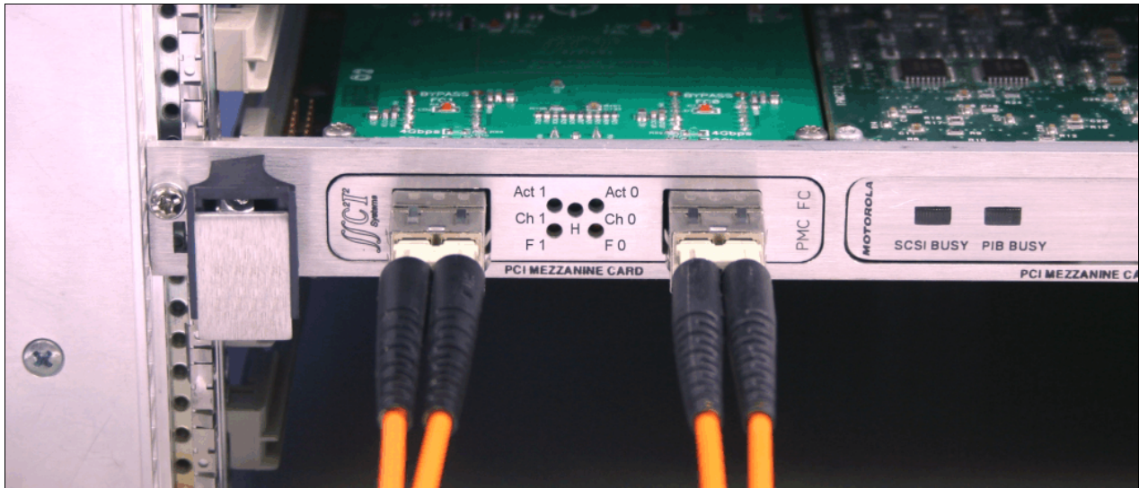
Figure 7 : FC Adapter with Duplex LC Connectors Attached
