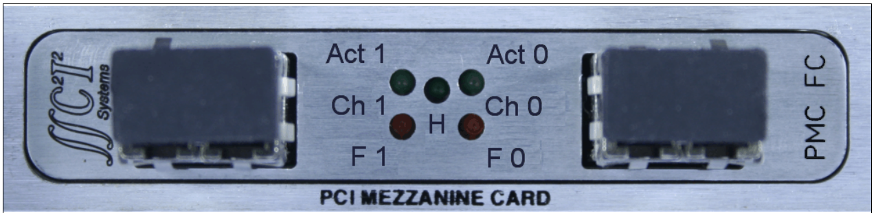
Figure 2 : Front Panel Indicators
