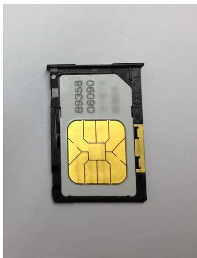
3. Insert the cradle to the Arctic. Make sure the cradle slides to the rails in the connector. Push the cradle all the way in until it stops.
