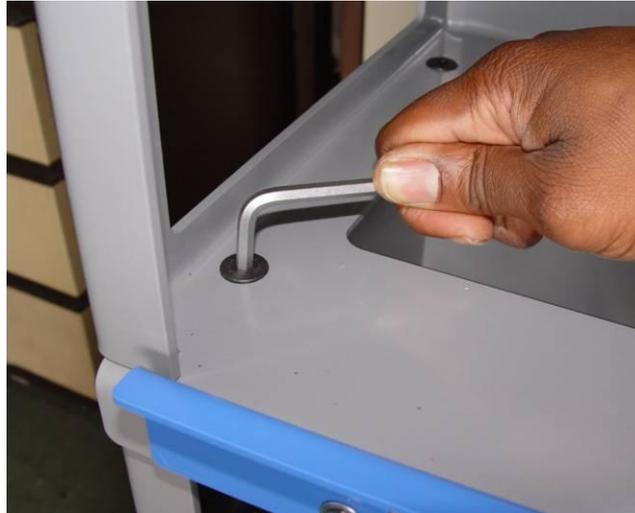
**Figure 9-5: Battery Housing module mount**
