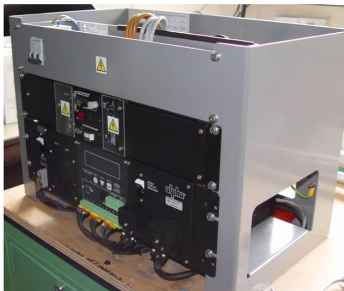
**Figure 3-5: UPS Housing Module**
