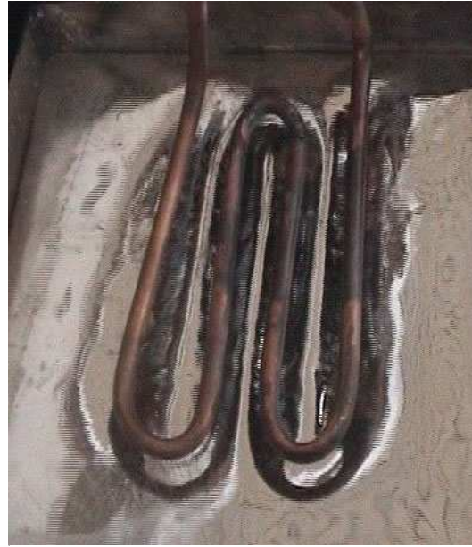
Figure 2.49: 40 kHz alternating current of 50 A in the four copper turns give rise to a ditch in the liquid metal. The metal ditch radius is 0.5 cm deep, to be compared with (2.37).
