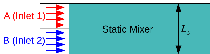
Figure 2.113: Mixing of a fluid of species A with a fluid of species B in a straight channel.
