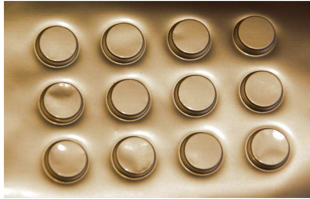
Figure 2.100: Blisters created by deep-drawing of a laminate.
