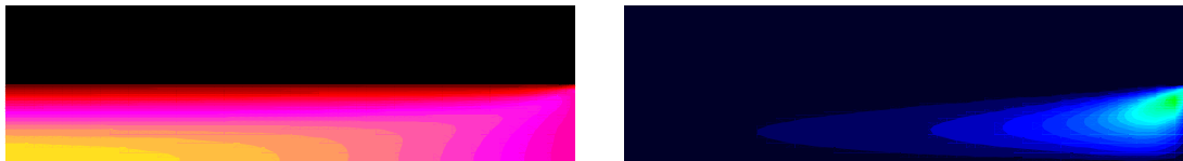
Figure 2.144: Velocity-distributions in axial (a) and radial (b) directions along the reactor; the lighter the color, the higher the velocity.
