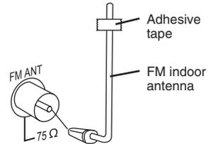
Tape the antenna to a wall or column, in a position with least amount of interference.
