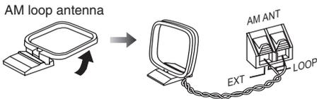
Stand the antenna up on its base. Keep loose antenna cord away from other wires and cords.
