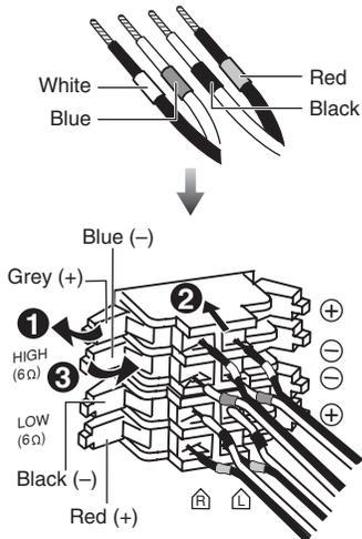
Cords with white and blue tags are for high frequency. Cords with red and black tags are for low frequency. **Incorrect connection can damage the unit.**
