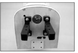
This is the distance that engine should be bolted to the motor mounts. Use a center punch or large diameter sharpened nail to mark the engine mounting bolt hole locations onto each motor mount. Remove the engine and remove the motor mounts from the firewall.
