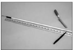
Starting from the threaded end, measure the 30cm metal pushrod back to 10-15/16" from the threaded end. At this point make a 90<sup>o</sup> bend. Trim the short bent end to a length of 3/8".
