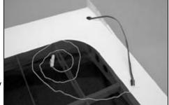
Since it is easily viewed through the top of the wing, align the servo accurately within the servo bay opening. Use pieces of masking tape to hold the servo tray in its final, correctly oriented position. Using the pre-drilled mounting holes in the servo tray as guides, drill four 1/32" dia. guide holes through the sheeting in the bottom of the wing.
