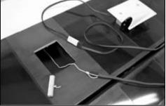
Pull the servo lead fully out of the exit, leaving no slack in the aileron servo bay. Remove the string from the servo lead and use a piece of tape to hold the lead to the wing for now.
