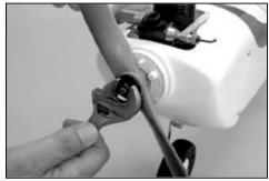
Note that it fits into the recess in the spinner backplate. Adjust the prop as needed until the spinner cone completely seats. Tighten the propeller nut firmly, locking the prop in place. Slip the spinner cone in place and secure it to the backplate with the two provided screws - snug these screws firmly but don't over-tighten them.
