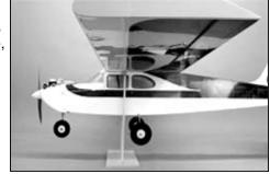
Some engines are considerably lighter than others and it may be necessary to use stick-on lead weights to get the model to balance. Since the KADET SENIOR ARF has so much wing area, adding such weight will do little to effect its flying ability. The best place to install lead weight is in the bottom of the cowl, just ahead of the nose gear strut. Make sure the weights are firmly attached to the cowl to ensure that they will not come loose in flight.
