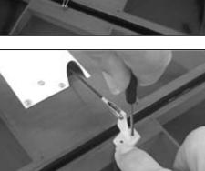
To secure the metal R/C link to the nylon control horn, cut a short length (about 1/4") of medium fuel tubing and slip it over the R/C link, onto its two arms. Attach the R/C link to the control horn and then slide the fuel tubing forward to the connection. This ensures that the R/C link will not be easily dislodged from the control horn - a very good safety practice for all such connections.
