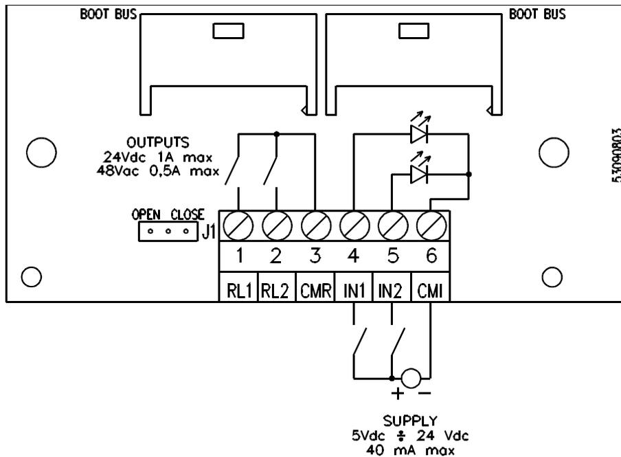
It is possible to connect 1 card (2 inputs / 2 relays) in the motherboard on the BOOT connector .
