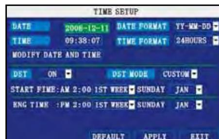
Figure 5.2 Configure DST settings
