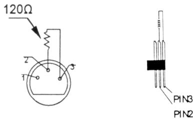
Termination reduces signal errors and avoids signal transmission problems and interference. It is always advisable to connect a DMX terminal, (Resistance 120 Ohm 1/4 W) between PIN 2 (DMX-) and PIN 3 (DMX +) of the last fixture.
