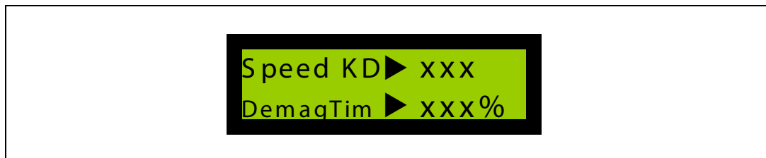
Figure 26. Configuring the speed regulator tuning derivative term: demagnetization time
