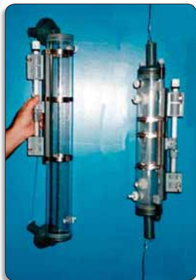
▲ Niskin deep water sampler
