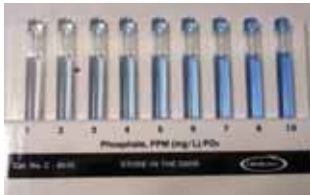
▲ Phosphate color comparator, high range
