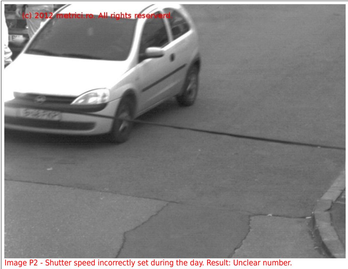
For guidance, depending on the relative travelling speed of the vehicle, we recommend the following minimum values for the shutter speed:
