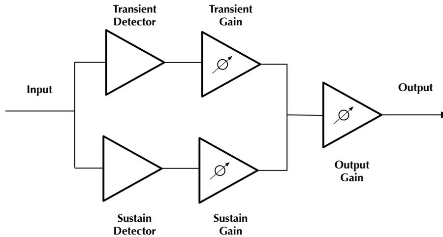
**Figure 3.1: TransientControl Block Diagram**
