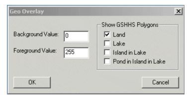
In order to create a Map Overlay the image has to have projection information. After creating the map overlay you can merge it into the image using *Multi* – <u>Overlay Image</u> (select the image first and then click on the Overlay icon on toolbar). Both the background and foreground pixel values of the overlay images can be selected.
