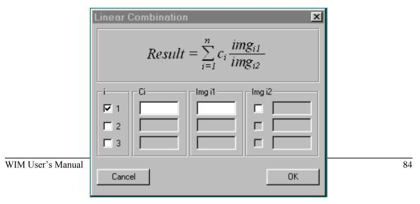
By either selecting or not selecting the second image, each term is either a an image multiplied by a coefficient or a ratio of two images multiplied by a coefficient. Images are selected by their sequence number (see <u>List of Images</u>). The resulting image is always a 4-byte-per-pixel float image.
