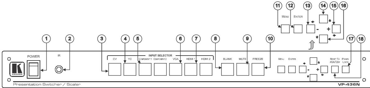
Figure 1: VP-436N Presentation Switcher/Scaler Front Panel
