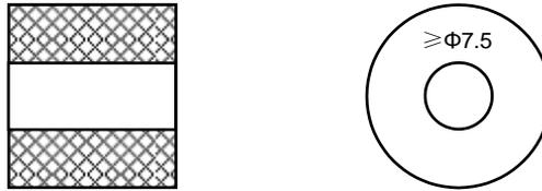
**Fig.7. 8mm sealing ring**
