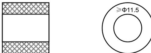
**Fig.9. 12mm sealing ring**
