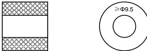
**Fig.8. 10mm sealing ring**
