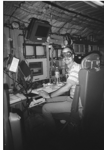
LabVIEW goes aloft. Gary works on a LabVIEW-based laser wavelength controller for an airborne LIDAR system aboard an Air Force C-135.
