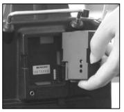
Different transmitters have different RF module connecting types. Therefore, before you purchasing our X8 system, you must make sure which one is suitable to your transmitter. The most popular Transmitters include Futaba and JR. But not all of them have isolate RF module and connect in the same way. Please read the instruction carefully and select right type.
