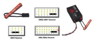
Binding is a process make the receiver known which one is his master. After bound, the receiver will only connect to that RF Module or Transmitter.
