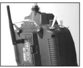
Mount removable antenna and screw it into the connecter at the back of ASSAN's X8 2.4GHz RF Module. Finger tight only.
