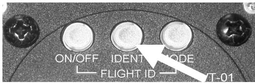
If required by the ATC, press the IDENT key (middle of the 3 keys of the transponder)
