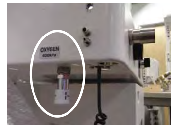
Additional High Pressure Outlet
