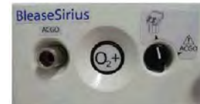
Auxiliary Common Gas Outlet
