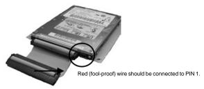
(Attention! Make sure that the reu (1001-proof) wire on the hopon capie should be connected to PIN 1 of the hard drive as shown below.)
