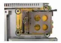
Step 2: Unload the part from another side of the PC. Then fix the PCMCIA card on the bolts and Fix the PCMCIA Card with screws.
