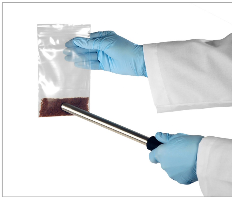
Figure 5. Sampling with the FlexIR through a thin plastic bag is possible due to the weak near-infrared signature of polyethylene.
