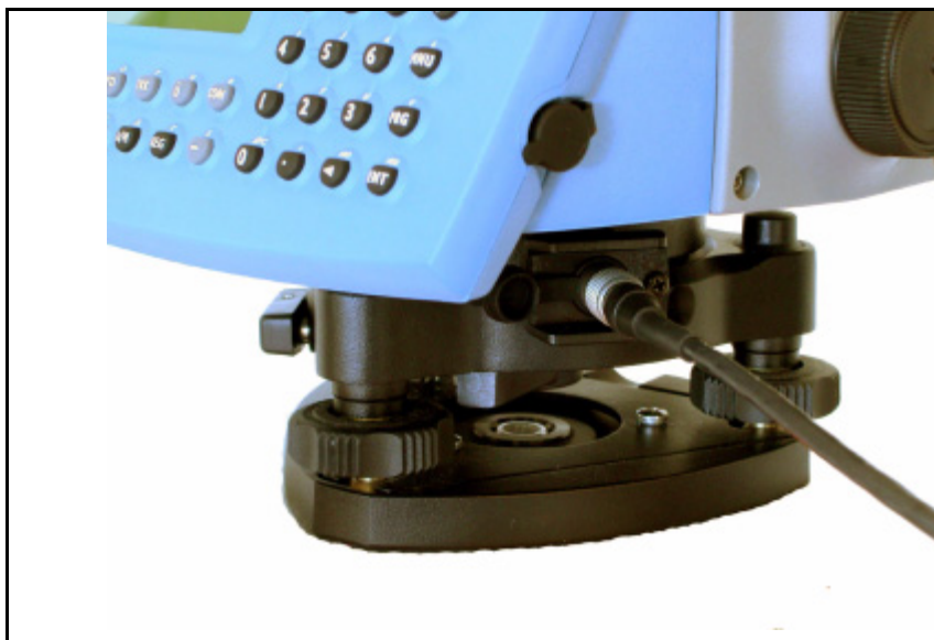
Figure 2.4 Connecting the external battery to the instrument.
