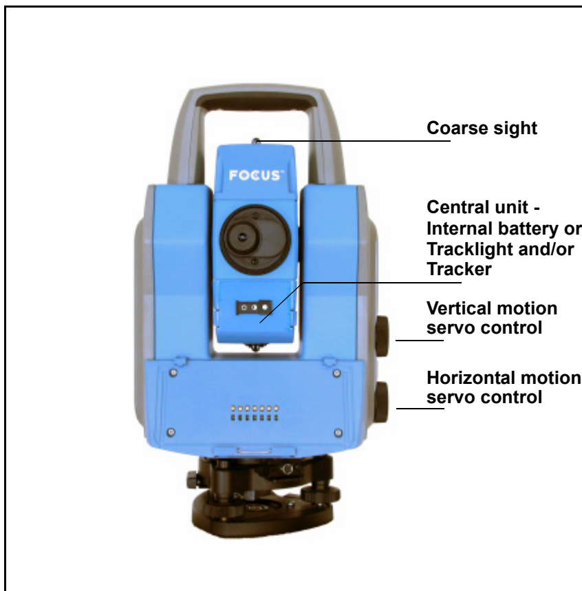
Figure 2.2 FOCUS 10 instrument shown from the operator side (back).
