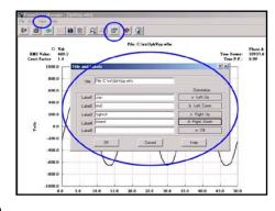
Normally, the scale of a display is set automatically by PSM to give the best size presentation of the data. However, when doing "before" and "after" comparisons, it is best to have identical vertical scales, otherwise a small "after" number may appear
