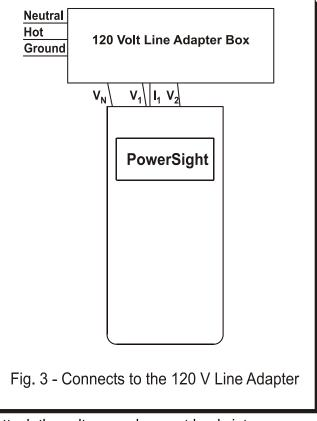
socket and then attach the voltage and current leads into PowerSight. Each lead is labeled to eliminate errors in connections.
