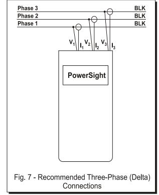
Please Note: Do not connect the V<sub>N</sub> input to anything when measuring in phase-phase measurement mode. This may affect the measurements associated with individual phases.
