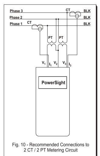
onto each of the primary currents directly, PowerSight must be operating in the 2 Current Probe mode of operation (see the <u>Phase-Neutral vs Phase-Phase vs 2 Current Mode</u> section).
