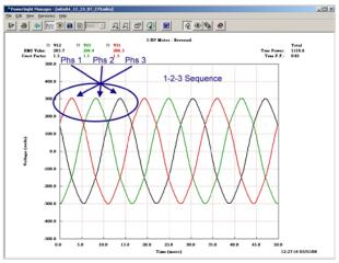
correct. Some utilities deliver power in that sequence and sometimes a motor will be connected in that manner to make it spin "backwards". An order of 2-1-3 or 1-3-2 is the same as 3-2-1, the reference point just starts in a different place (for instance 2-1-3 is a portion of the continuing sequence of 3-2-1-3-2-1).
