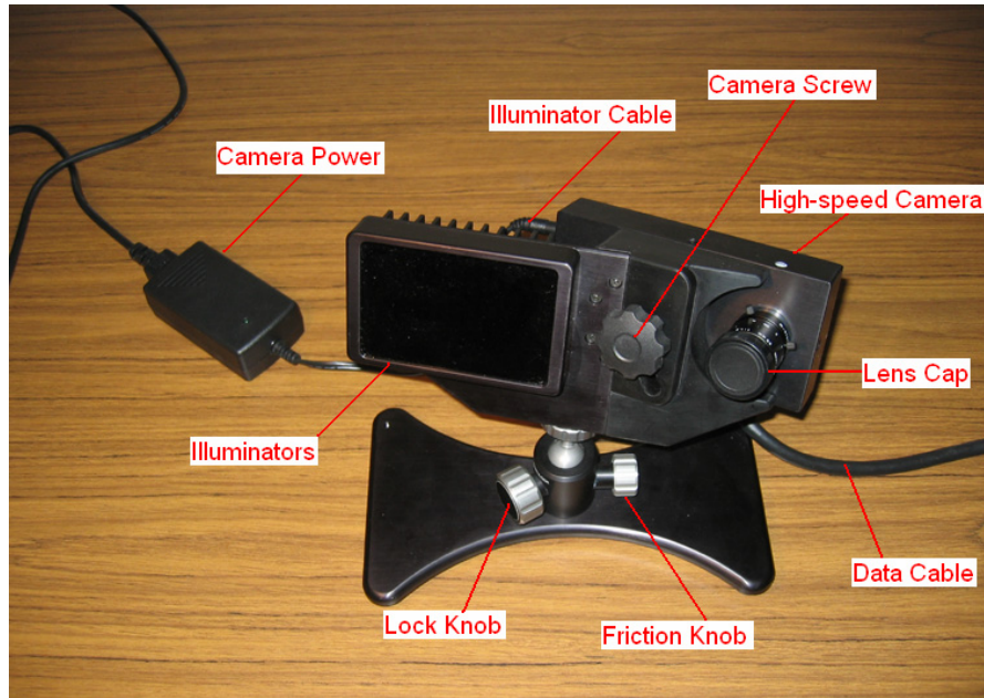
Figure 4-1 EyeLink 1000 Desktop Mount Components
