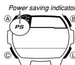
When turned on, the Power Saving function enters a sleep state automatically whenever the watch is left in an area for a certain period where it is dark. The table below shows how watch functions are affected by the Power Saving function.
