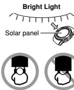
The electricity generated by the solar panel of the watch is stored by a rechargeable battery. Leaving or using the watch where it is not exposed to light causes the battery to run down. Make sure the watch is exposed to light as much as possible.
