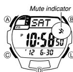
The button operation tone sounds any time you press one of the watch's buttons. You can turn the button operation tone on or off as desired.
