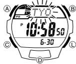
1. In the Timekeeping Mode, hold down (A) until the city code starts to flash, which indicates the setting screen.
