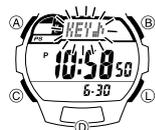
1. In the Timekeeping Mode, hold down (A) until the city code starts to flash, which indicates the setting screen.
