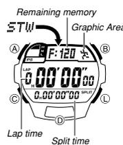
The 1/100-second stopwatch can measure elapsed time and lap/split times. Stopwatch times are stored in memory.
