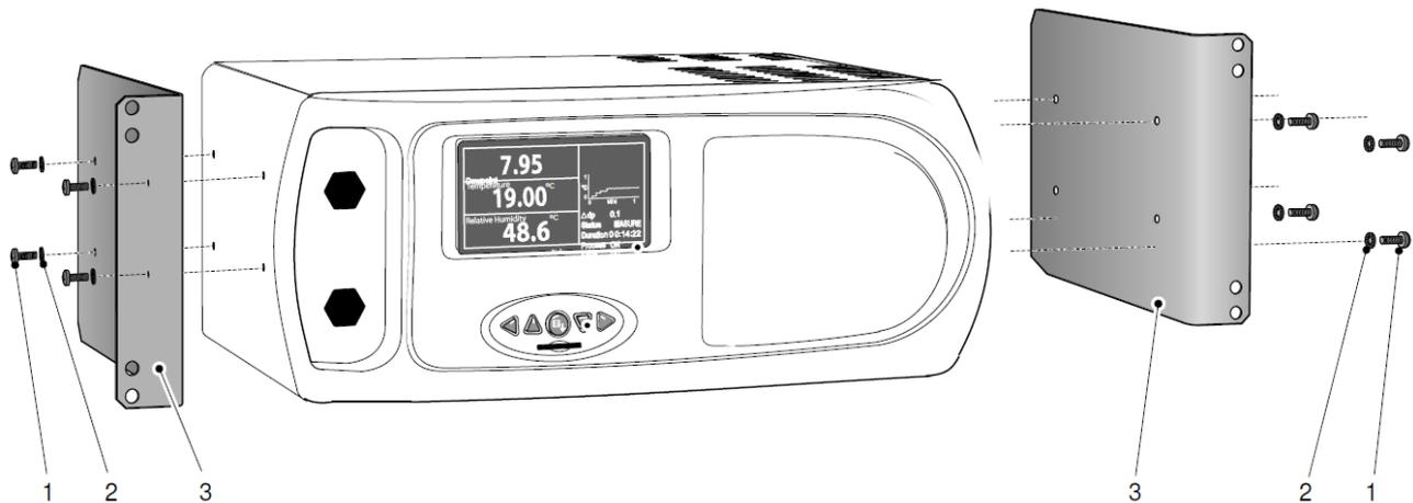
**Figure 2.2** Conversion of Horizontal to Rack Mount
