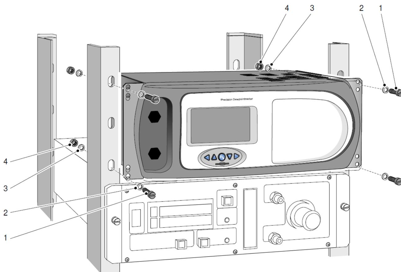
**Figure 2.3** Rack Installing Method
