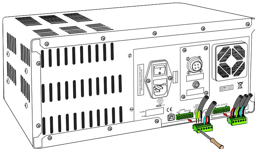
**Figure 2.6** Alarm and Analog Output Connectors
