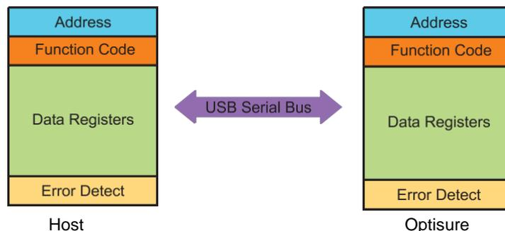
**Figure F1 - Modbus Connection**
