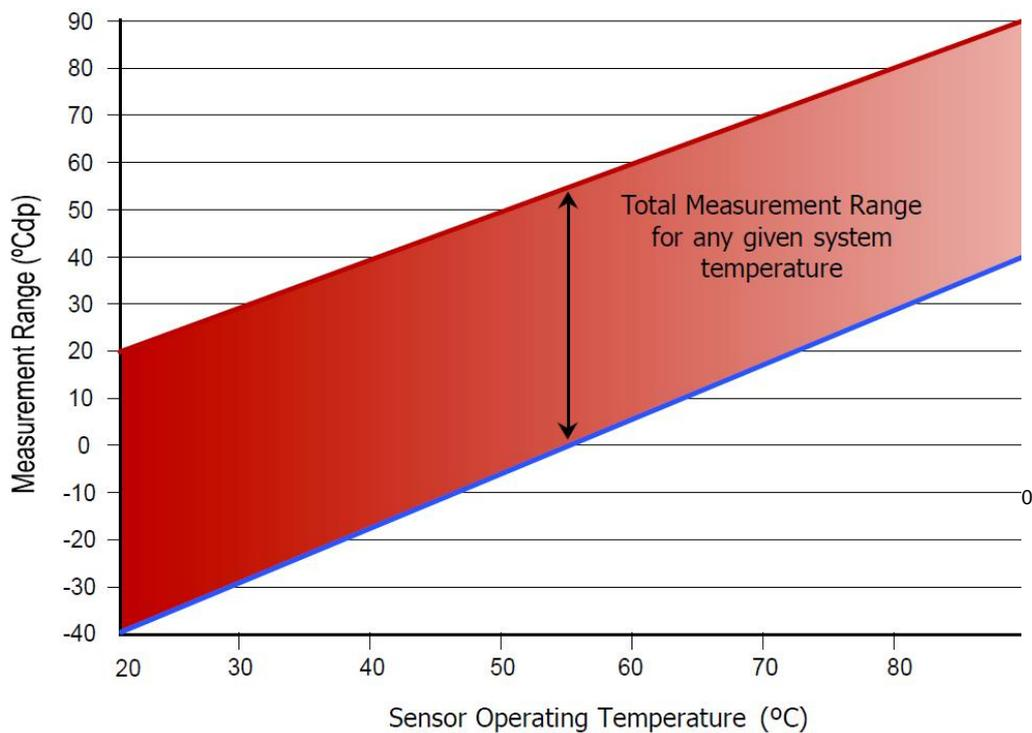
**Figure A.2** Optisure Remote Measurement Range
