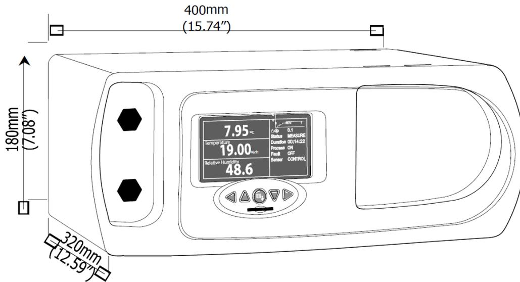
**Figure A.1** Optisure Remote Dimensions
