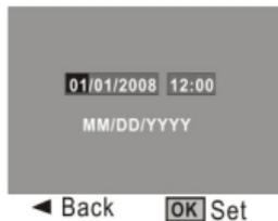
To change the date and time, use the Direction key: Up or Down to adjust, Right key to move the cursor, OK key to confirm, then OK key to Exit setup mode.
