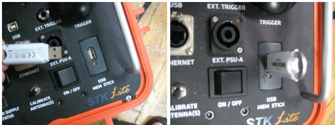
FIGURE 6 – INSERTING USB MEMORY STICK INTO READER
