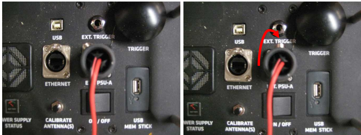
FIGURE 2 – PLUGGING IN THE 3-STEP CHARGER
