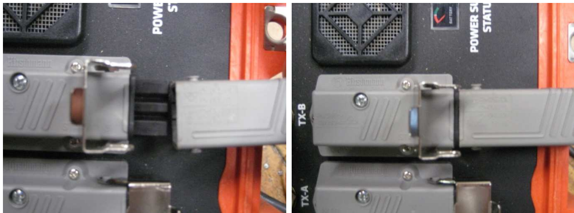
FIGURE 8 – CONNECTING MATS (TX CHANNEL)
