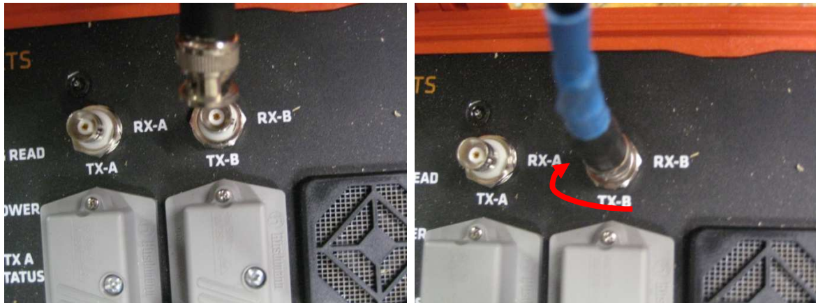
FIGURE 7 – CONNECTING MATS (RX CHANNEL)
