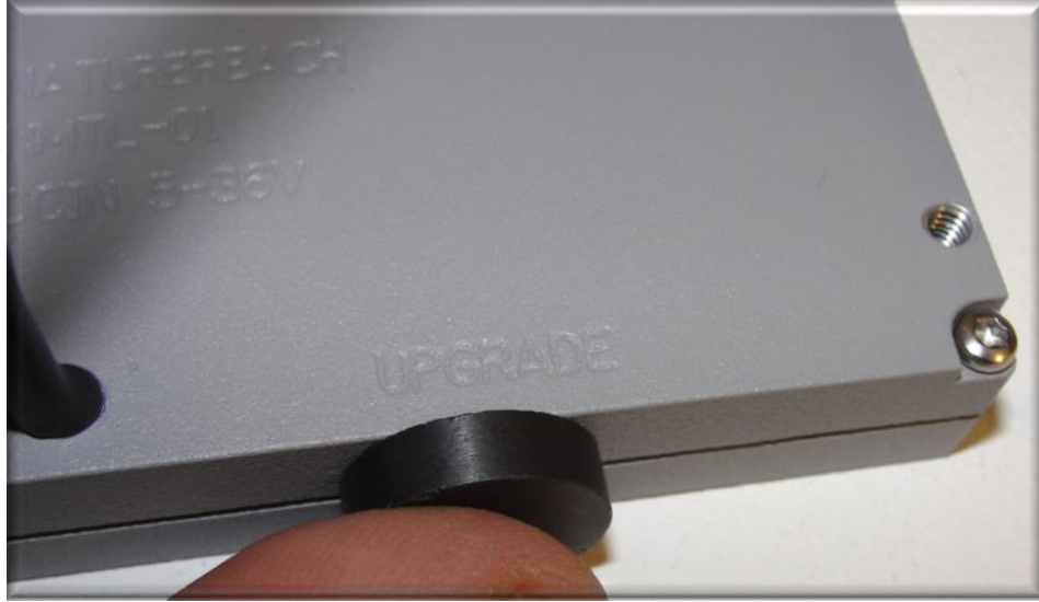
Figure 17 Positioning the earth magnet for firmware programming mode
