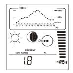
The upper section will display the 24-hour future tide height, as a percentage of highest tide height. In the TIDE RANGE mode, the total tide **range** will be displayed in feet or meters. This is the lowest tide height subtracted from the highest tide height; thus the range will not necessarily be the highest tide (for example, a high tide of 8.4 m and a low tide of 1.0 m is a tide range of 7.4 m).
