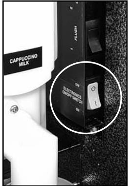
4. Open the front door of the machine. Switch **on** the mains electricity supply and the electronics on/off switch (figure 5) located on the switch panel.
