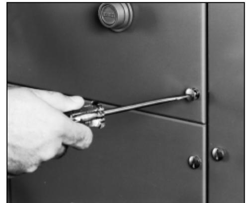
Figure 50: Loosening Captive Quarter-turn Fasteners
