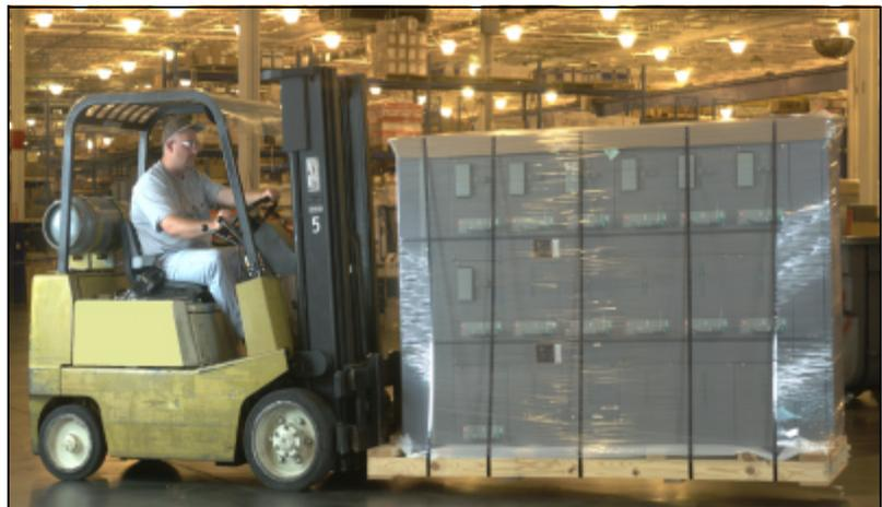
**Figure 2: Moving the MCC with a Fork Truck**
