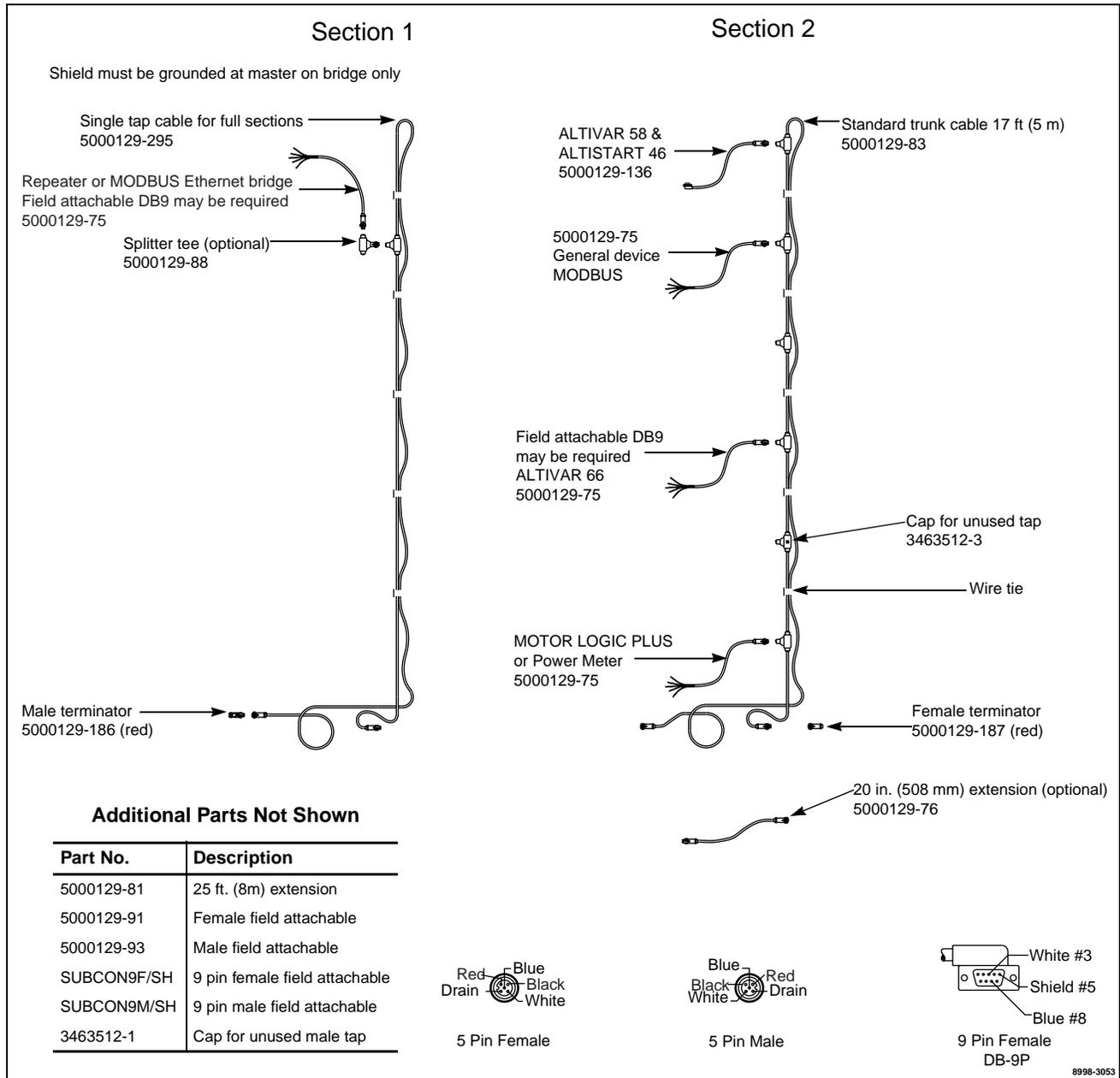
Figure 33: Typical Cabling Scheme for MODBUS 4-Wire
