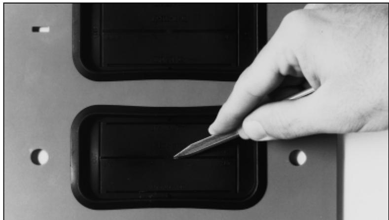
**Figure 64: Cutting the Vertical Wire Trough Grommet (when supplied)**
