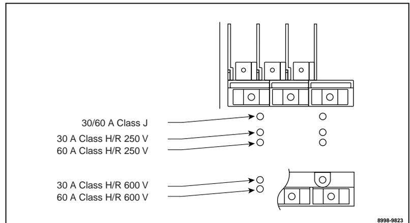
**Figure 32: Size 1 and 2 Fuse Clip Location**
