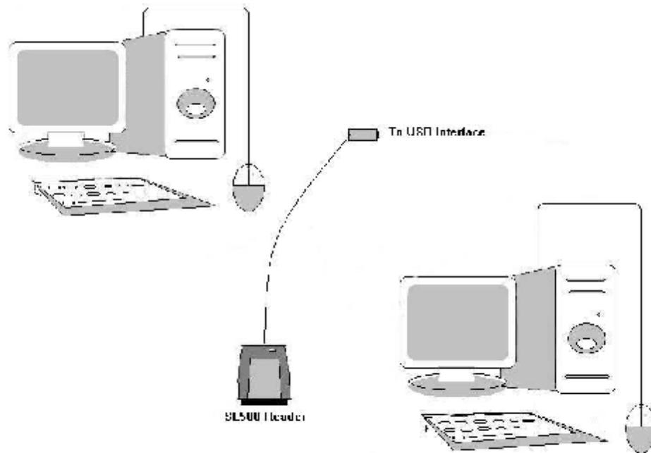
GZ500-USB Reader is USB bridge to COM. Connect GZ500 to the USB port of PC, after installing the driver will come out a virtual COM, the operations hereafter are as same as GZ500-RS232.
