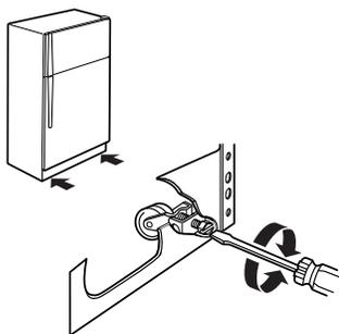
3. Open both doors again to make sure that they close as easily as you like. If not, tilt the refrigerator slightly more to the rear by turning both leveling screws to the right. It may take several more turns, and you should turn both leveling screws the same amount.
