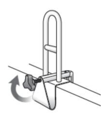
DO NOT over-tighten the clamp on fiberglass and or porcelain tubs as it may crack or damage them.
