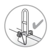
WARNING: The safety rail may require tightening from time to time. Check periodically and tighten again when needed.
