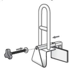
3. Turn the screw in a "clockwise" direction to begin to secure the back plate to the rail as shown in Fig 2 below:
