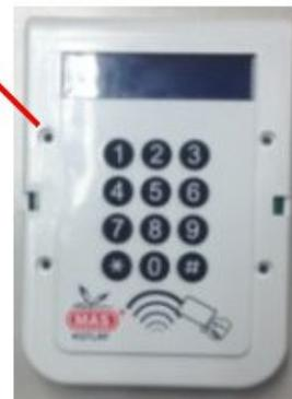
Fix the device on the wall by replacing back cover
