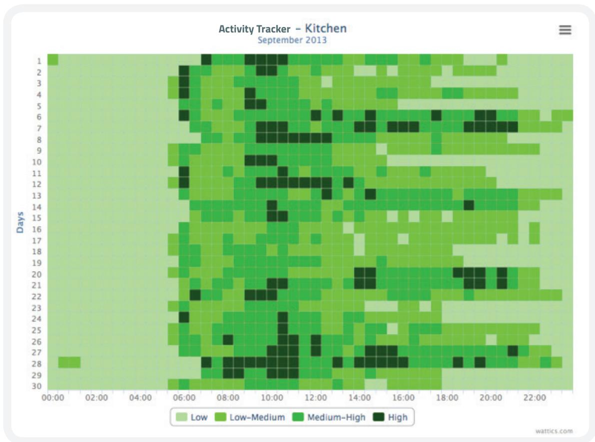
Such a data representation allows quick evaluation of habits/patterns in power consumption and when load demand is at its maximum. Periods of high power activity can often appear at unexpected times, and prove to be sources of wastage. For instance a piece of equipment left on overnight will generate a dark green tint which will be immediately visible on the Activity Tracker.
