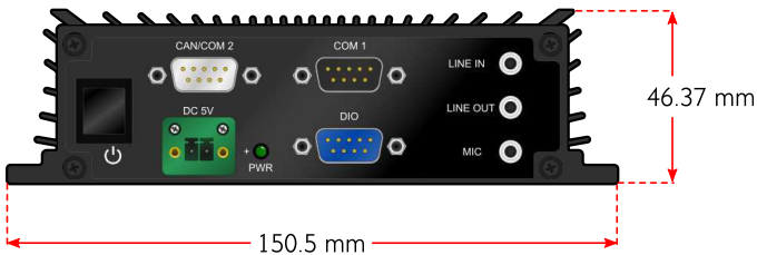
Figure 2: Dimensions of the AMOS-800 (front view)
