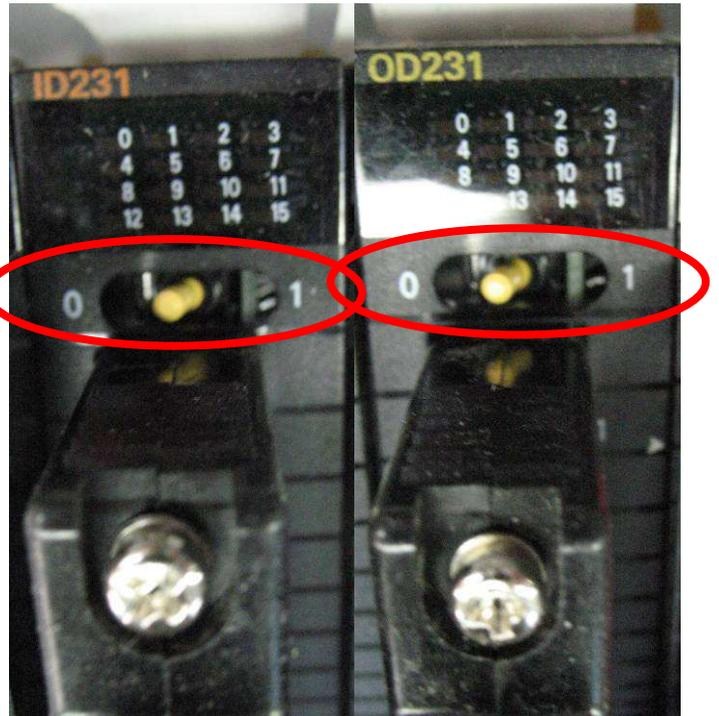
For example, to visualize the input, you must verify the "DEL2" on the ID231 module with the switch on the right (1).
