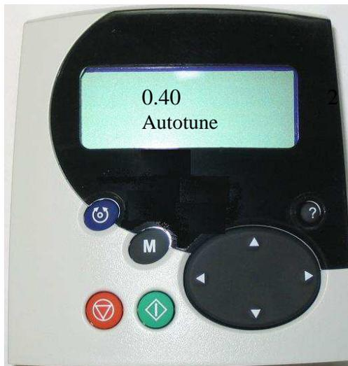
Put "2" in the parameter 0.40, place the elevator in controller inspection mode, use a jumper between +A and PCH or control inspection (put a jumper between +A and ISR to activate control inspection) press ▲ or ▼ on the control inspection circuit and hold it until parameter 0.40 indicates 0. The test is now complete. The dephasing value will be in parameter "0.43" and the current gains will be in parameters "0.38" and "0.39". **Save in the drive.**
