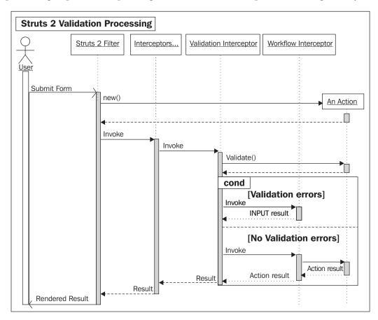
Here, we're representing the user action of submitting a form in the sequence diagram. This (in simplified form) causes the Struts 2 filter to instantiate the appropriate action class, indicated by the **new()** message. The rest is (I'd imagine) largely self-explanatory.
