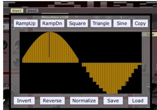
Editing buttons: **Invert** flips the polarity of the waveform; **Reverse** flips the waveform in time; **Normalize** adjusts the amplitude of the waveform so that the largest value is at full scale.
