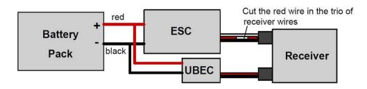
Suggestion: You can use a sharp screwdriver to take the pin (with red wire) out from the BEC connector of the ESC, and then insulate it with a bit of electrical tape for further use, so you needn't cut the red wire by this method.
