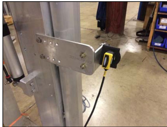
Pic #50B: Sonar Photo-Eye Installed
